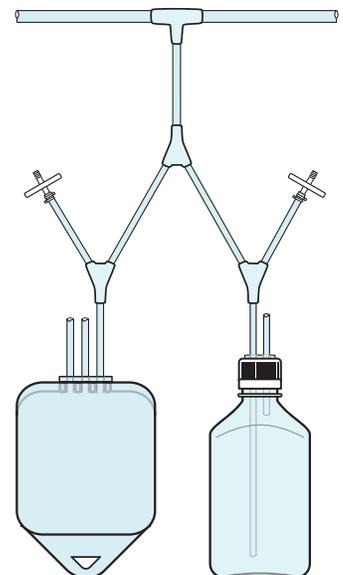
Molded manifolds can be used with a variety of containers, vessels, biobags, etc. for batch filling and sampling needs
