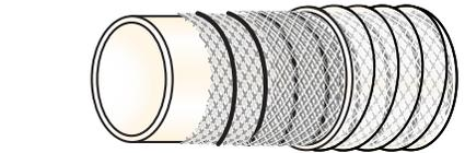
**APSW – 4-Ply, Wire-Reinforced, Mandrel-Wrapped Silicone Suction Hose:** Polyester Mesh Fabric; Spiral Wrapped; Smooth or Convoluted O.D.; 8 stock sizes from 1/2" I.D. up to 4" I.D.
