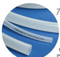
dvantaFlex TPE (thermoplastic elastomer) tubing addresses the need for a flexible, translucent, sterilizable, moldable, heat sealable, and weldable biopharmaceutical tubing for fluid processing. AdvantaFlex maintains its physical properties following sterilization processes, resists kinking, remains translucent for visible product flow, and does not become gummy.
